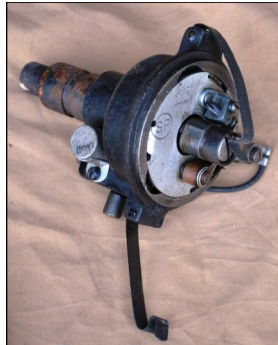
#2 A 1932 Ford model B distributor. The word "good" marked on box.
