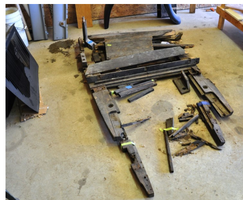
This rotted wood was all that Sandy Scott had for patterns when building the body.
