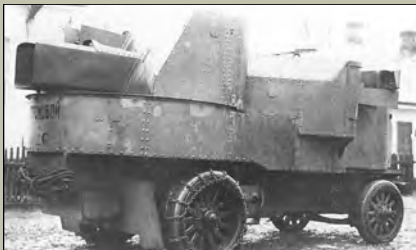
An WWI army variant Garford-Putilov armoured car named "Gromoboi" pictured after repair in 1916. Extra armour has been added to protect the machine guns. Note the chains on the rear wheels to try and improve off-road ability.
