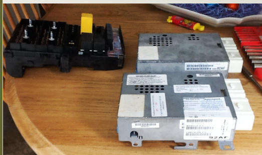
New BCM (bottom) old BCM (top). The BCM is mounted in the fuse/relay block to the left. The whole assembly fits under the dashboard.
